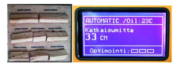
When the log's end passes the optical sensors, the optimization starts. The length left is optimized accorded to the selected settings. The three optimization options symboles represent the 3 last pieces of wood passing to the saw (see pictures on the right).
