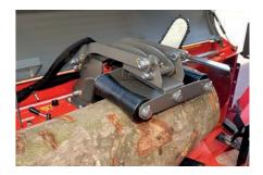
The hydraulic log clamp enables logs of all sizes to be sawed effortlessly.
