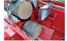
The log landing plates ensure that even the shortest cut logs land neatly into the splitting groove.
